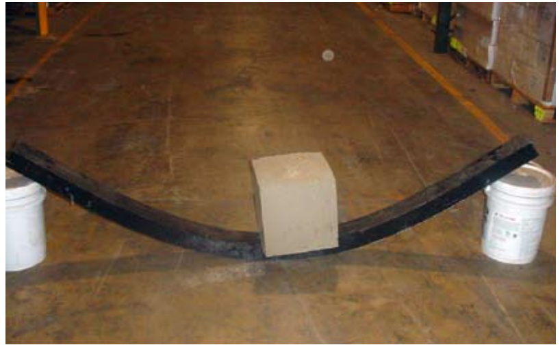
Photograph illustrates the flexibility of WaboCrete II
