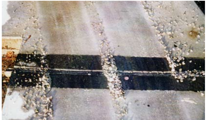
Abrasive Test - WaboCrete II after 100,000 load repetitions
